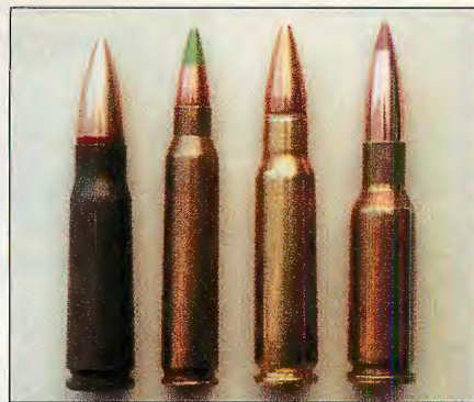
Shown from left are the 7.62x39mm, 5.56x45mm, 6.8x43mm Rem. SPC, and the 6.5mm Grendel. The 6.8mm out shoots them all.
